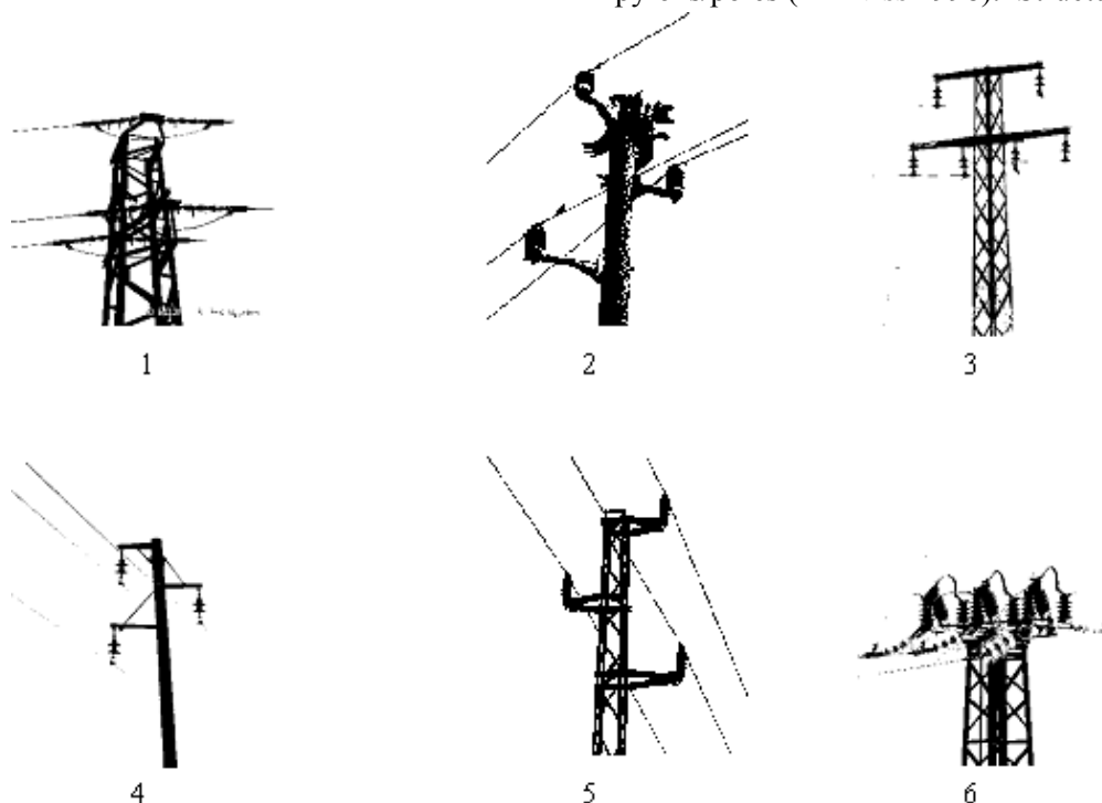
Fig. 4. Different 20 kV pole configurations.
